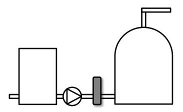
S38 Unit should be fitted on the cold feed to where the water is heated, after any pumps or tanks
